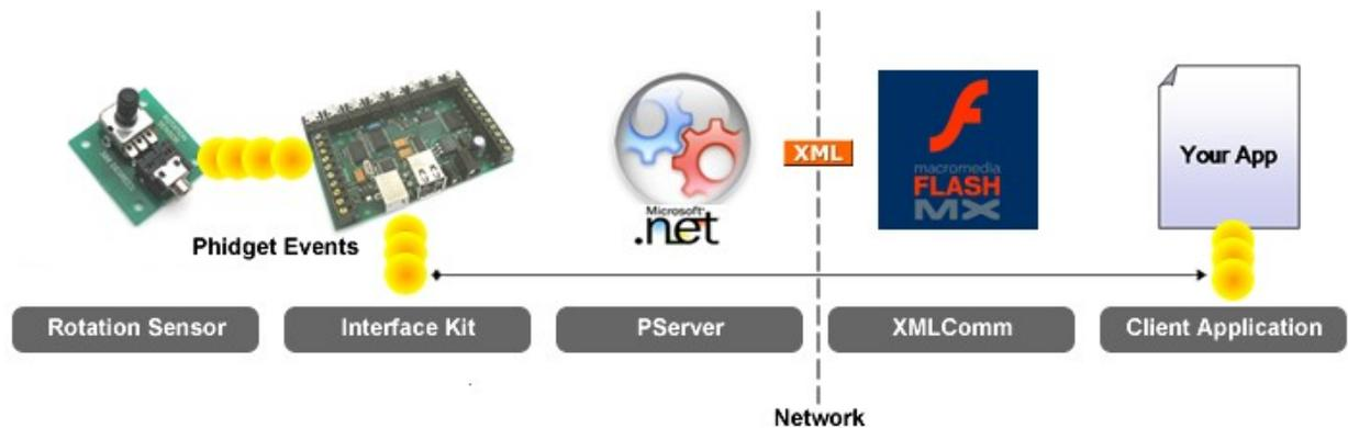
**Figure 1:** Phidget Server event flow diagram
