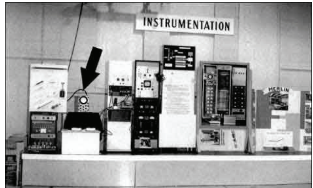
Figure 1: The BNL Instrumentation Division's Visitor Day display from 1958 showing the oscilloscope and electronics which ran the Tennis For Two video game (below arrow). [5]
