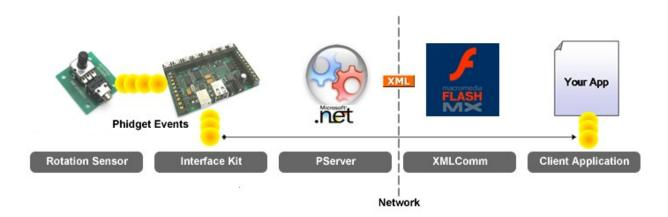
Figure 1: Phidget Server event flow diagram
